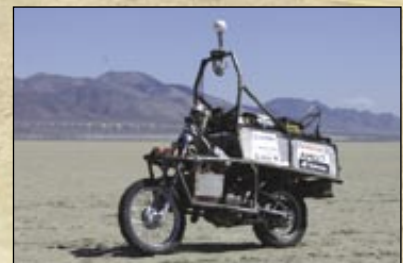
GHOSTRIDER ran unassisted for 20 miles at a time in desert testing.
